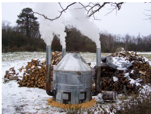
A new producer in Amherst County takes advantage of winter weather and cool temperatures to produce his first batch of natural hardwood lump charcoal. Photo by:
